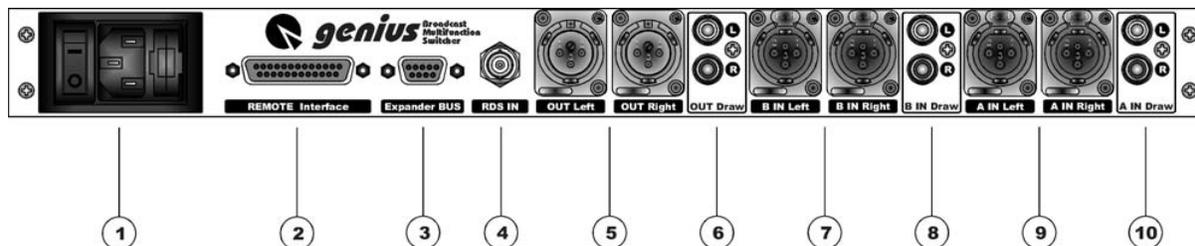
**ON/OFF switch:** it switches on the equipment, the led inside shows the status of the equipment. If the led is off and the switch is ON please check the power supply wire and the PWS protection fuse integrity
