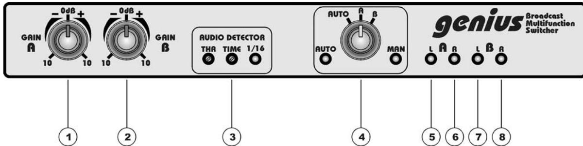
**GAIN A:** Potentiometer setting the signal level on the A input, it controls  $\pm 10$  dB.
